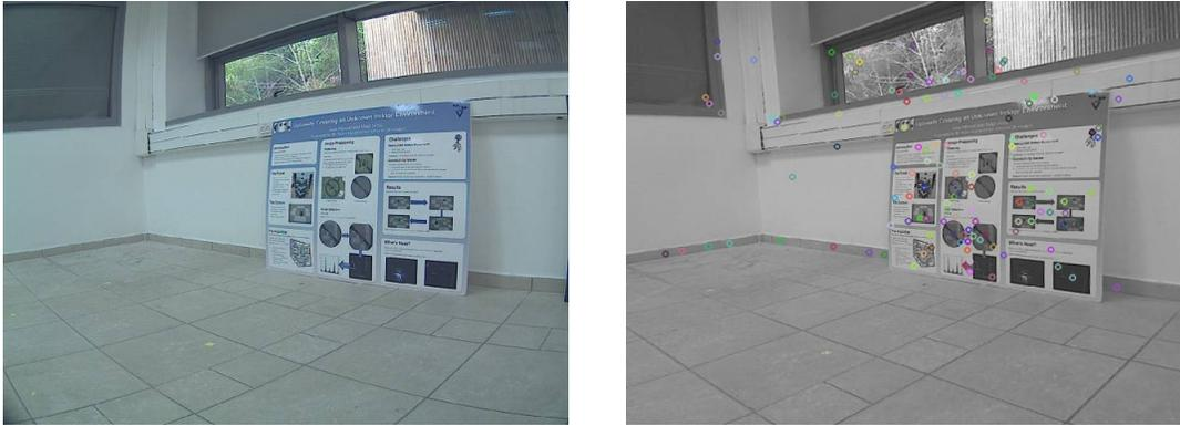
Figure 5: An original distorted image from the camera & its undistorted unidentical twin
