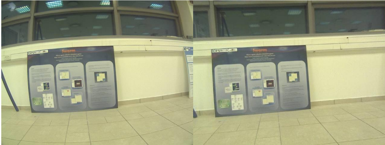
Figure 4: to the left is the original image, and to the right is the undistorted one.
